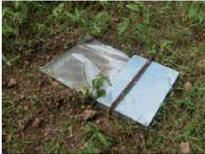
Photo 3.01 – Soil and water collector
