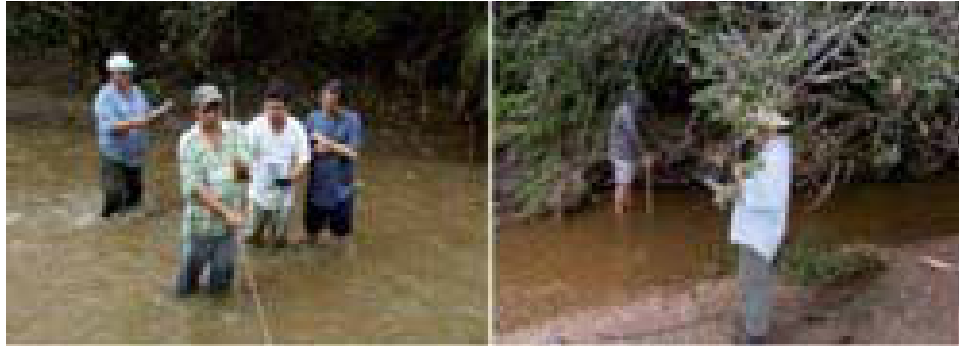
Photo 2.12 – Discharge measurement at key-curve calibration stage.
