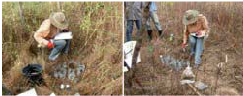
Photo 2.11 – Infiltration essays using “Beerkan” method
