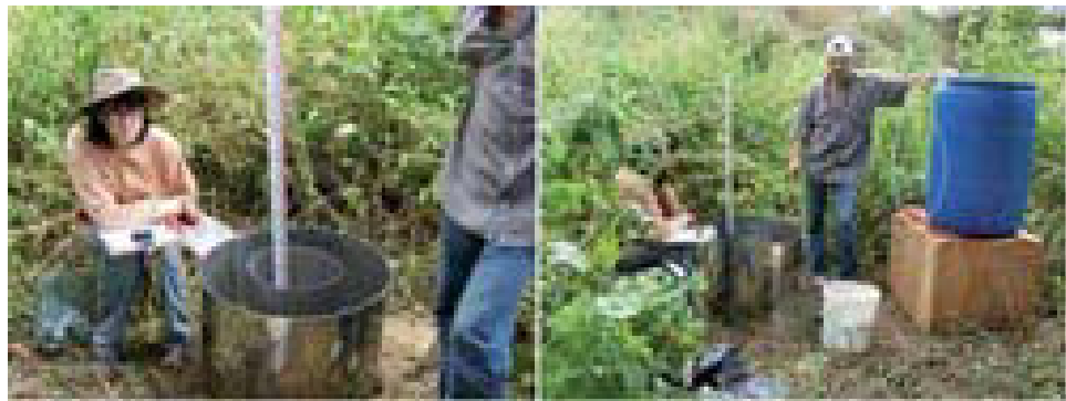
Photo 2.10 – Infiltration essays using concentric rings
