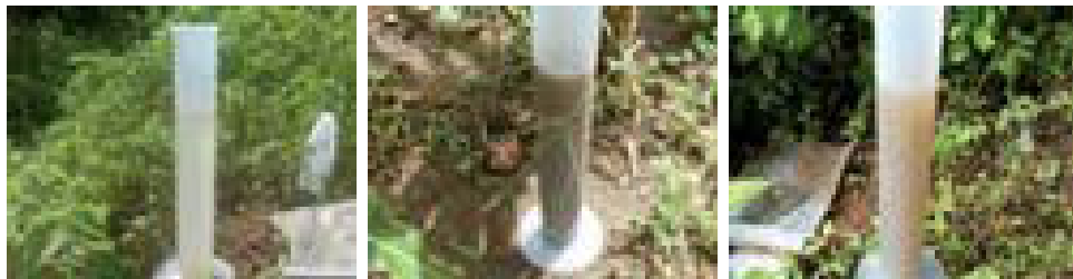
Photo 3.07 – Turbidity difference noted in beakers at volume measurement
