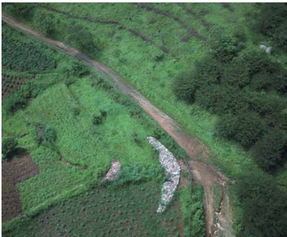
Photo 10 – Air View of Cangati River HMB showing Vegetation Remains Row, Surrounding Stone Barrier, Successive Dam and Contour Line Cultivation Techniques.
