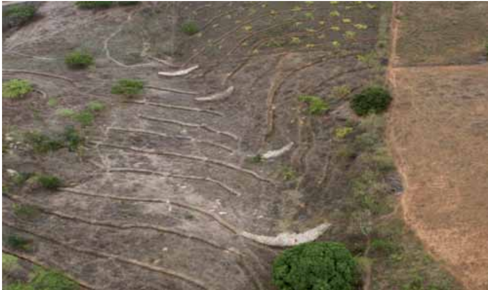
Photo 4 – Air view of a Series of Dams and Surrounding Stone Barriers in Dry Period (Summer), in a HMB assisted by PRODHAM
